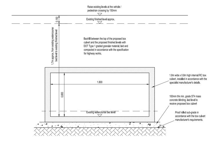
Typical Detail Through Proposed Box Culvert
